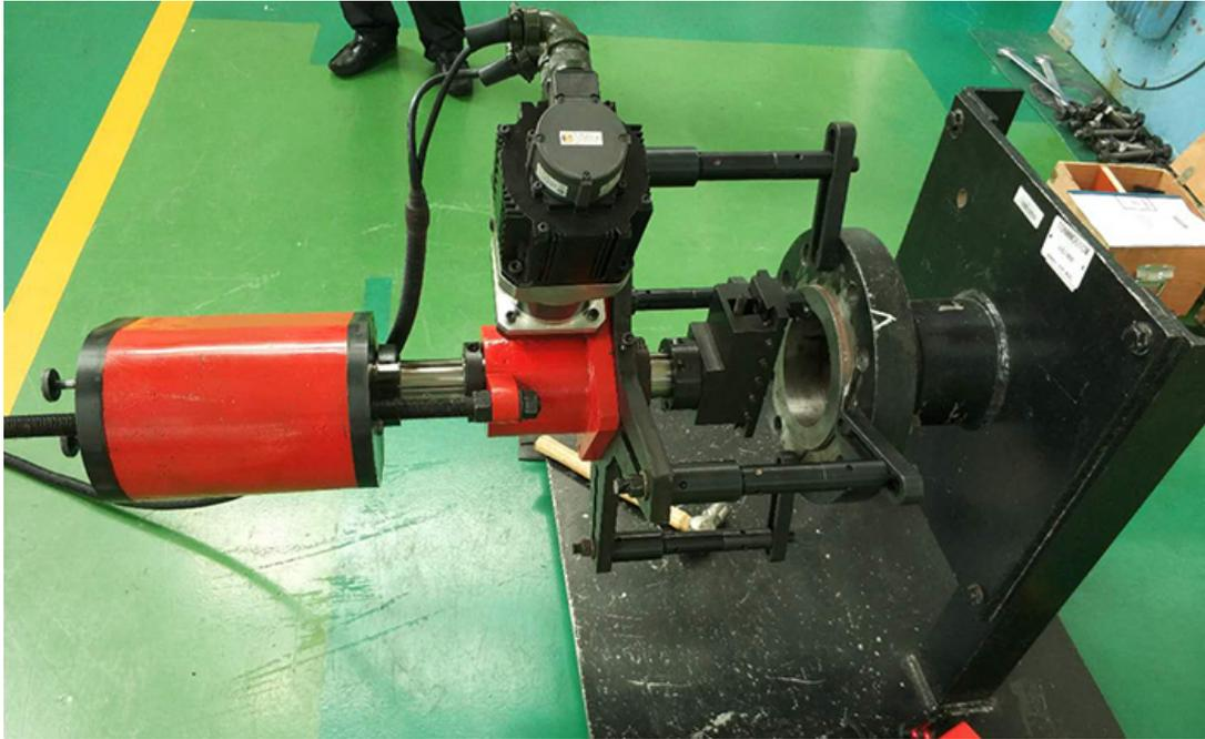
Our TDF400-A portable valve repair machine is a multi-functional equipment. The standard accessory is a turning machine. The optional accessories enable TDF400-A to finish different works.
